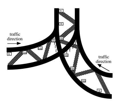
Here is a picture of two portways merging into one portway. The boxes with control information are placed along the inside of the left rails. The letter "n" occurs where the portway indicates "normal (not approaching a merge or turn or all porter exit)"; flanges are in their retracted position. The letters "lm" occur where the portway indicates "on the left branch approaching a
