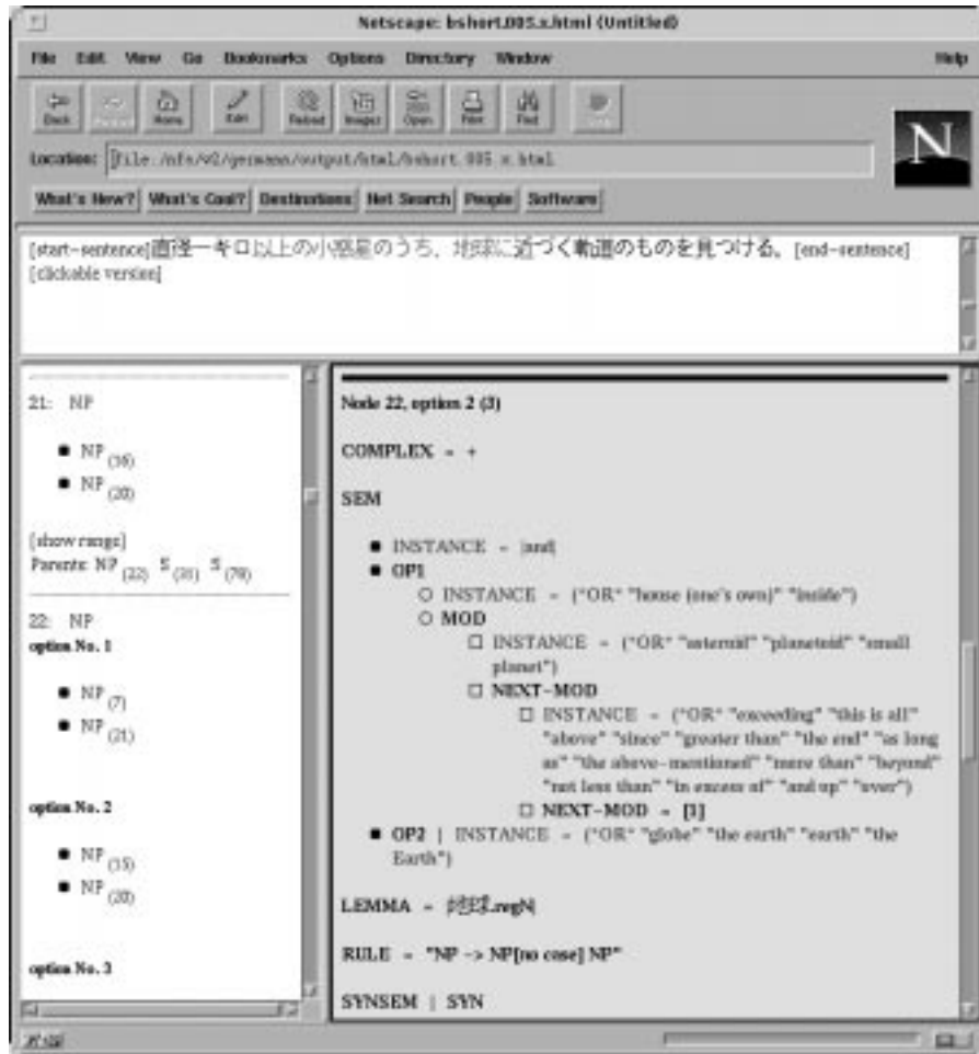
Figure 5: Sample screen. The top frame displays the original input text, which serves as an index to the parse sequence in the lower left frame. The category labels and node numbers in the lower left frame are hyperlinks. A click on a category label will cause the browser to display the feature structure(s) associated with that node in the frame on the right. A click on a node number will lead to the respective node within the parse sequence.
