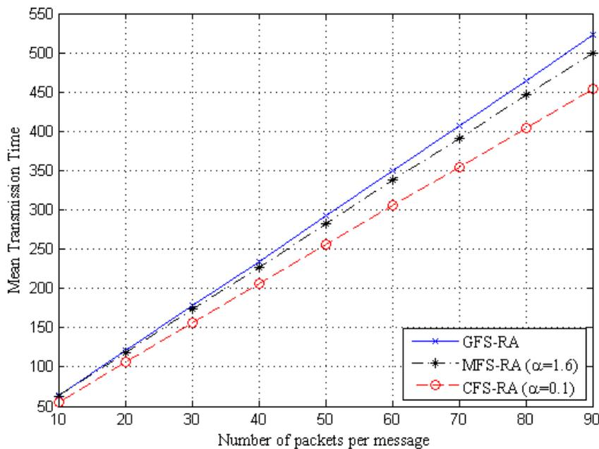
Fig. 4.8 Mean Transmissions Time (MTT) Performance of all the algorithms as a function of number of packets per message on Network II, destination set = {7,9,12,13}
