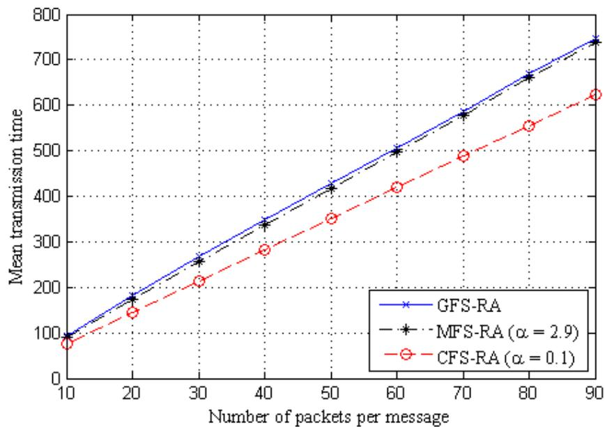
Fig. 4.7 Mean Transmissions Time (MTT) Performance of all the algorithms as a function of number of packets per message on Network I, destination set = {8,15,17,21}
