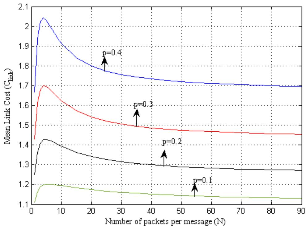
Fig. 4.6 Variation of mean link cost ( $C_{link}$ ) with  $N$  for different erasure probabilities  $p$
