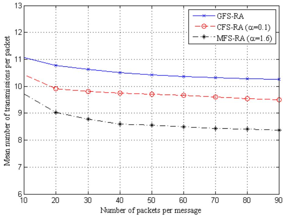
Fig. 4.5 Mean Number of Transmissions per packet (MNT) Performance of all the algorithms as a function of number of packets per message on Network II, destination set = {7,9,12,13}
