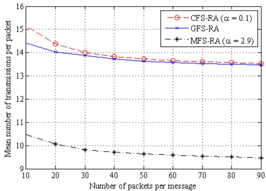
Fig. 4.4 Mean Number of Transmissions per packet (MNT) Performance of all the algorithms as a function of number of packets per message on Network I, destination set = {8.15,17,21}
