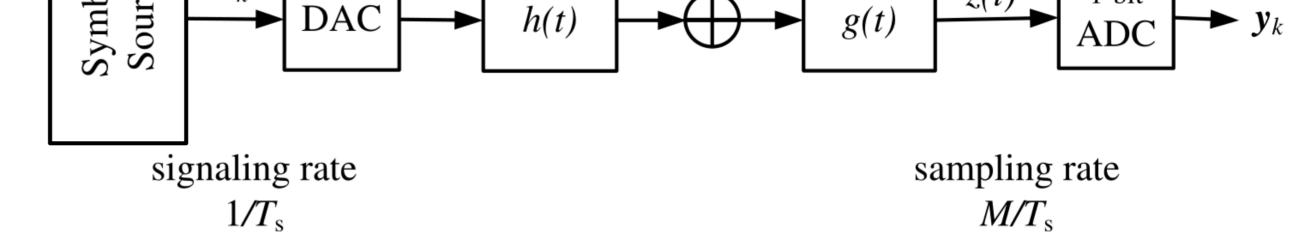
System Model with a 4-ASK symbol source, AWGN finite memory channel, matched filters and 1-Bit quantization & oversampling at the receiver
