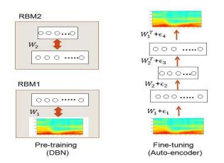
Fig.1. Left: Illustration of pre-training of the DBN that consists of two RBMs used in this work. Right: Illustration of fine tuning that produces the final deep auto-encoder.
