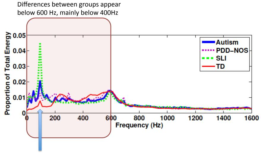
spikes of varying height near 100 Hz, possibly an electric hum harmonic
