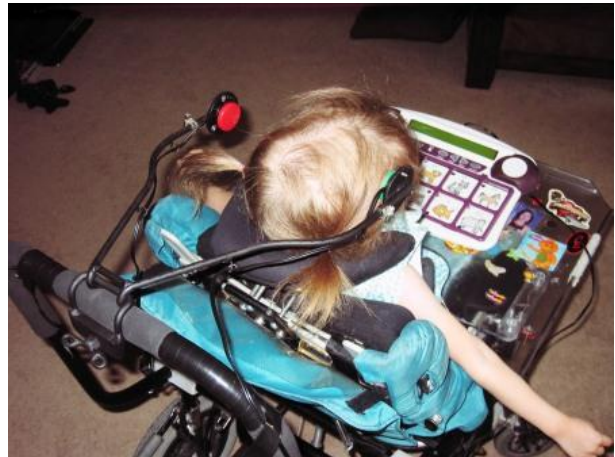
Figure 1: Example of a two-button head-switch mounted on a wheelchair. Image used by permission of the Tetra Society of North America.
