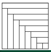
A submatrix is **monochromatic** if *f* is constant on inputs in the submatrix. A deterministic protocol computing f repeatedly partitions  $M_f$  into rectangles (submatrices) until every rectangle is monochromatic.
