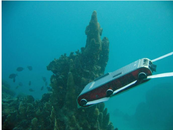
FIGURE 1.2. The second generation of the Aqua family of underwater robots.
