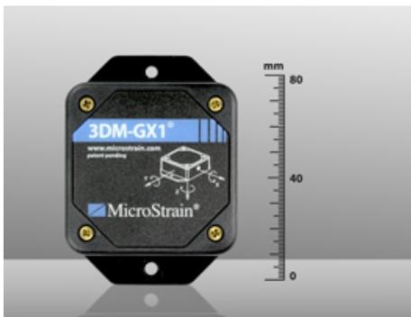
FIGURE 1.1. The particular IMU sensor that we are using, the MicroStrain 3DM-GX1, incorporates a MEMS (microelectromechanical system) accelerometer, gyroscope, and magnetometer.
