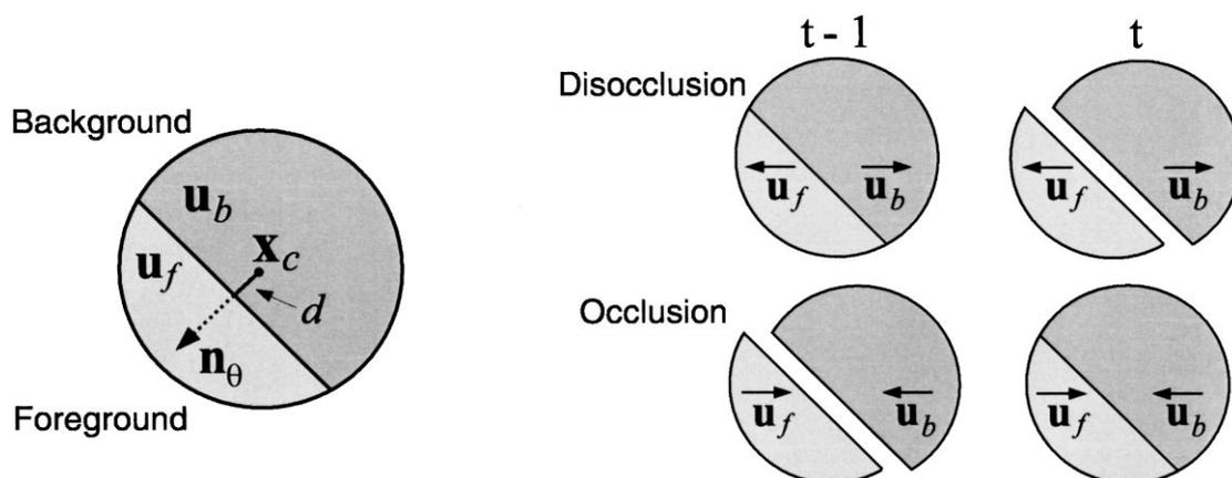
Figure 1. Model of an occlusion boundary, parameterized by foreground and background velocities,  $\mathbf{u}_f$  and  $\mathbf{u}_b$ , an orientation  $\theta$  with normal  $\mathbf{n}_\theta$ , and a signed distance  $d$  from the neighborhood center  $\mathbf{x}_c$ . With this model we predict which pixels are visible between frames at times  $t-1$  and  $t$ .
