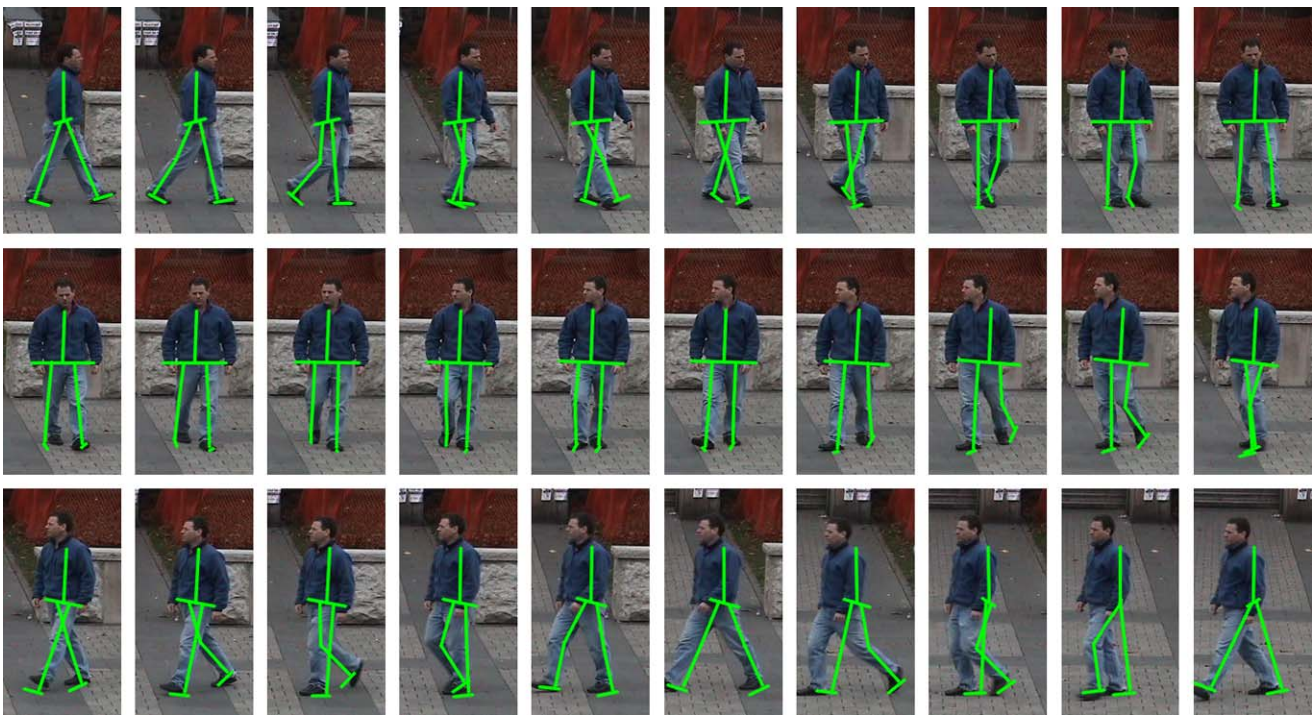
Fig. 14 (Color online) Cropped images showing every 5th frame of the MAP trajectory through an acceleration and sharp turn, starting at frame 200. The skeleton of the kinematic model is overlaid in green. The middle row corresponds to the shaded portion of Fig. 13
