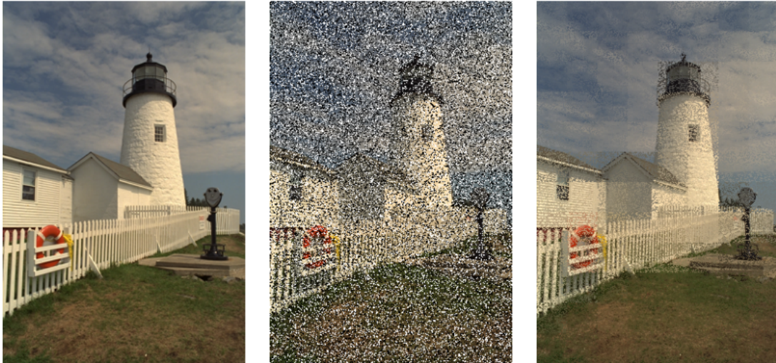
Figure 3: (left) The noiseless image of the lighthouse. (middle) The noisy image corrupted with the salt-and-pepper noise. (right) The output of RBF regression model that performs denoising.
