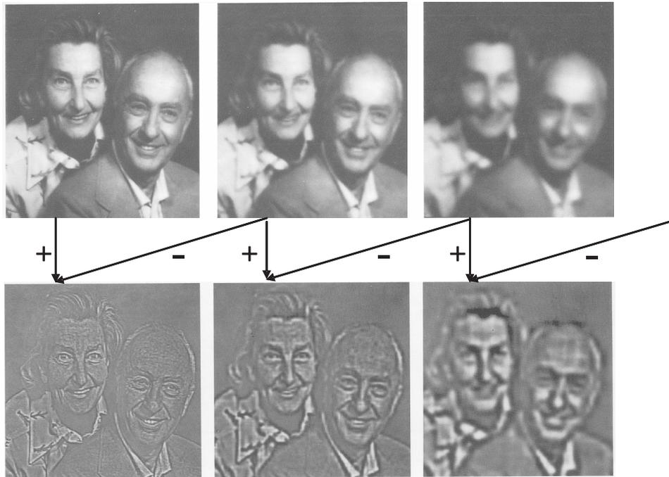
A Laplacian pyramid with four levels:
