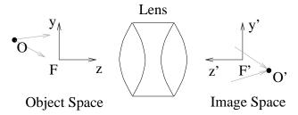
In general the ratio of focal lengths equals the ratio of the indices of refraction of the pre- and postlens material, that is f/f' = n/n' (eg.  $f \neq f'$  for eyes, but f = f' for most cameras). The index of refraction of a material is the ratio of the speed of light in a vacuum over the speed of light in that medium.
