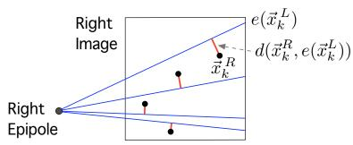
We could minimize the sum of squared epipolar distances  $d(\vec{x}_k^R, e(\vec{x}_k^L))$  for  $k = 1 \dots K$ . However, due to the normalization factor in (20), the objective function is not quadratic in the unknown F.
