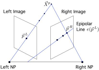
**Epipolar Line:** The scene point  $\vec{X}^p$  that projects to  $\vec{p}^L$  lies on a ray from  $\vec{d}^L$  through  $\vec{p}^L$ , but the position of  $\vec{X}^p$  on the ray is unknown. Importantly, the image of the ray can be shown to be a line in the right image, called the *epipolar line*,  $e(\vec{p}^L)$ .
