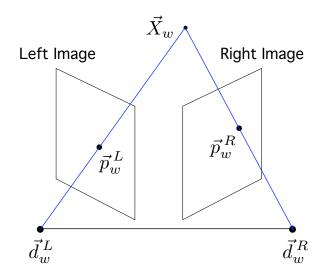
The 3D plane defined by  $\vec{p}_w^{\,R}$ ,  $\vec{d}_w^{\,L}$  and  $\vec{d}_w^{\,R}$ , has normal direction
