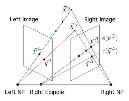
The epipolar line  $e(\vec{p}^L)$  depends on the position of the left image point. A different point,  $\vec{q}^L$ , generally produces a different epipolar line,  $e(\vec{q}^L)$ .
