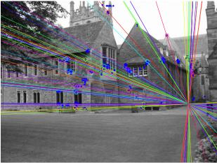
Here have choosen random colours to circle image features. The same colour is then used for the corresponding point in the other image, and also for the epipolar lines generated from these two points.
