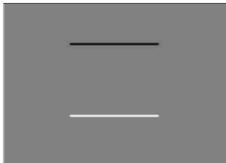
\frac{\partial f(x,y)}{\partial y} with [-1, 1]^T and correlation
