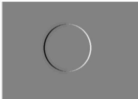
\frac{\partial f(x,y)}{\partial x} with [-1, 1] and correlation
