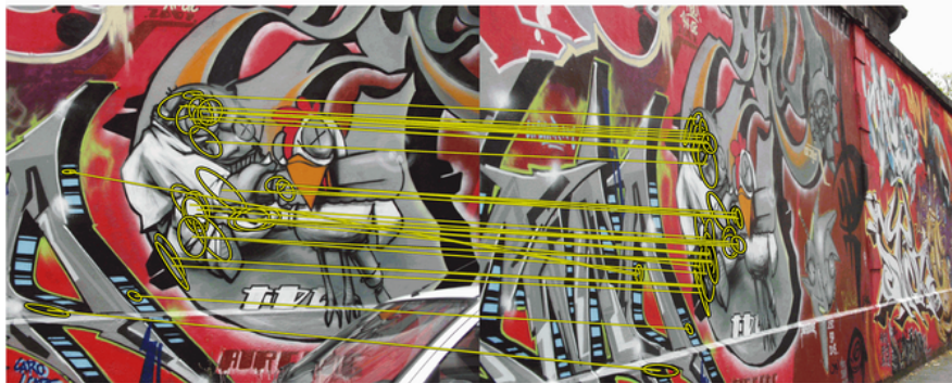
Figure: Lowe's interest point detector finds scale-invariant points that can be reliably matched across different images. (We will talk about how to do matching soon)
