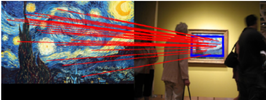
Figure: Lowe's interest point detector finds scale-invariant points that can be reliably matched across different images. (We will talk about how to do matching soon)
