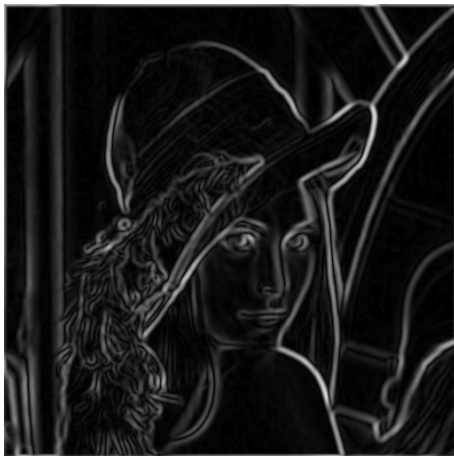
Figure: Canny's approach takes gradient magnitude
