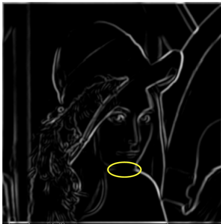
Figure: Problem with thresholding
