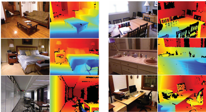
Figure: The NYUv2 dataset: RGB-D images collected with Kinect
