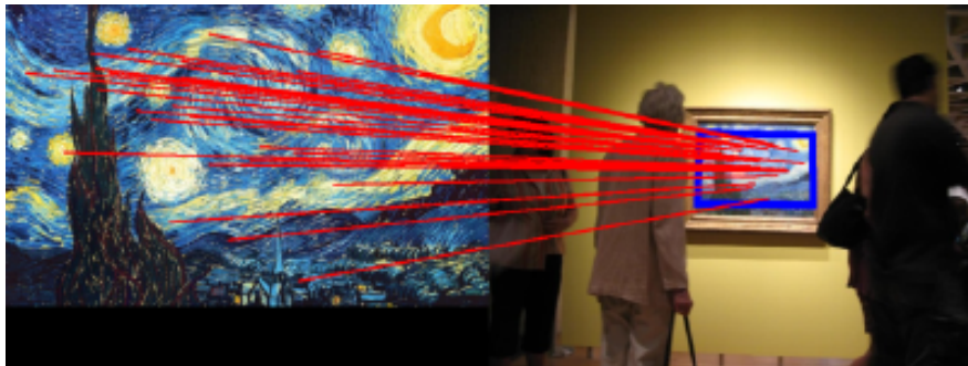
Figure: Lowe's interest point detector finds scale-invariant points that can be reliably matched across different images. (We will talk about how to do matching soon)
