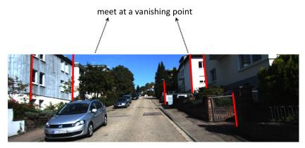
Figure: Extract "vertical" lines and compute vanishing point. How can we compute direction in 3D from vanishing point (if we have K)?
