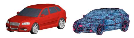
Figure: A CAD model is a collection of 3D vertices and faces that connect the vertices. Each face represents a small triangle. It typically has color.
