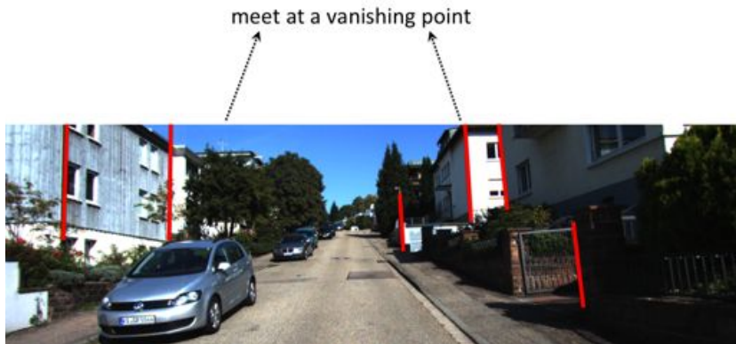
Figure: Extract “vertical” lines and compute vanishing point. How can we compute direction in 3D from vanishing point (if we have K )?
