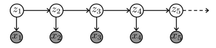
$p(\mathbf{z}_{1:T}, \mathbf{x}_{1:T}) = p(\mathbf{z}_{1:T})p(\mathbf{x}_{1:T} | \mathbf{z}_{1:T}) = \left[ p(z_1) \prod_{t=2}^T p(z_t | z_{t-1}) \right] \left[ \prod_{t=1}^T p(\mathbf{x}_t | z_t) \right]$
