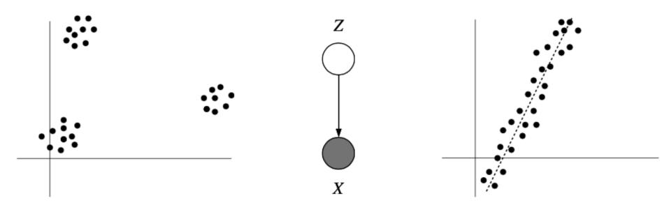
• You can think of factor models (such as factor analysis, PCA, ICA, etc.) as linear or nonlinear regression with missing inputs.
