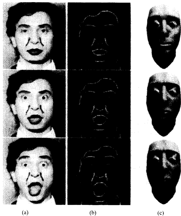
Fig. 7. Dynamic facial image analysis and expression resynthesis. Sample video frames with superimposed deformable contours tracking facial features; (a) intensity images with black snakes, (b) image potentials with white snakes. (c) Facial model resynthesizes surprise expression from estimated muscle contractions.
