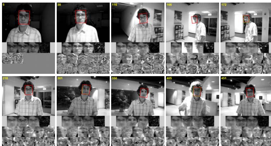
Figure 1: A person moves from dark toward bright area with large lighting and pose changes. The images in the second row shows the current sample mean, tracked region, reconstructed image, and the reconstruction error respectively. The third and forth rows shows 10 largest eigenbases.
