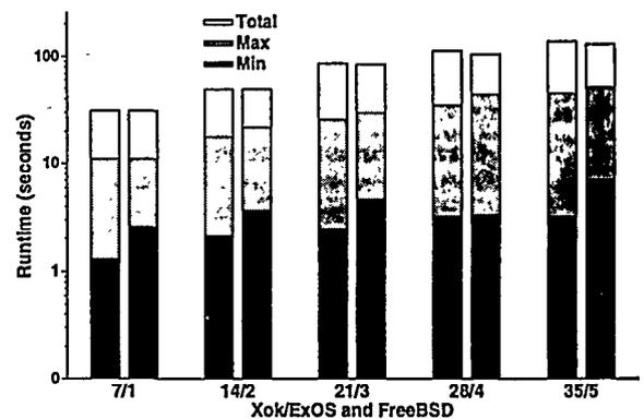
Figure 4: Measured global performance of Xok/ExOS (the first bar) and FreeBSD (the second bar), using the first application pool. Times are in seconds and on a log scale. *number/number* refers to the total number of applications run by the script and the maximum number of jobs run concurrently. Total is the total running time of each experiment, Max is the longest runtime of any process in a given run (giving the worst latency). Min is the minimum.
