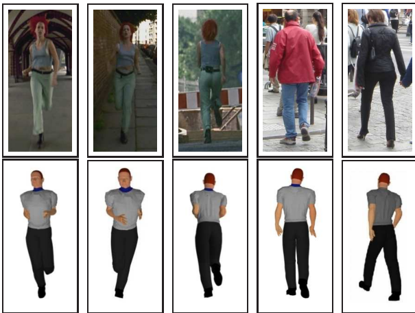
Figure 6. Qualitative 3d reconstruction results obtained on images from the movie ‘Run Lola Run’ (block of leftmost 3 images) and the INRIA pedestrian dataset (rightmost 2 images) [6]. (a) Top row shows the original images, (b) Bottom row shows automatic 3d reconstructions.
