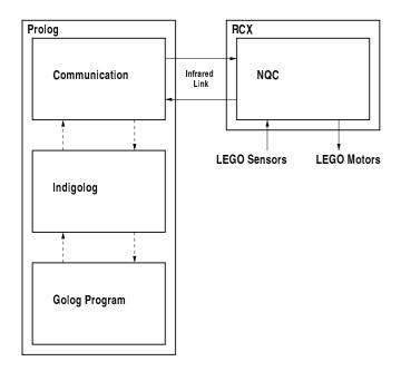
Figure 1. Idealised view of Legolog structure.
