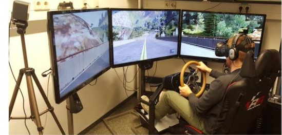
Figure 1: Experimental setup: Participants saw the game [21] either on the flat screens in front of them (traffic scene and a speedometer) or via a VR HMD (see in-cockpit scene in Figure 2).
