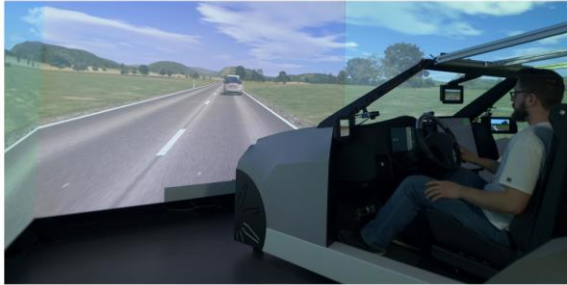
Figure 4: Fixed-base driving simulator of the Department Human Factors at Ulm University.
