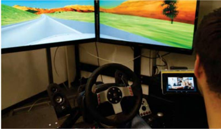
Figure 3: The driving simulator in which the study was conducted. The participant is watching a video while automation is activated.
