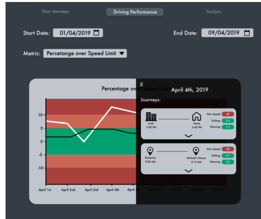
Figure 6: Driving performance of a driver over all their journeys between two chosen dates. The individual performance is also compared with the community average over the same timeline. The user has the option to choose between three separate metrics: percentage over the speed limit, weaving score, and drifting score. Clicking on any individual point on the graph shows the statistics for that day.
