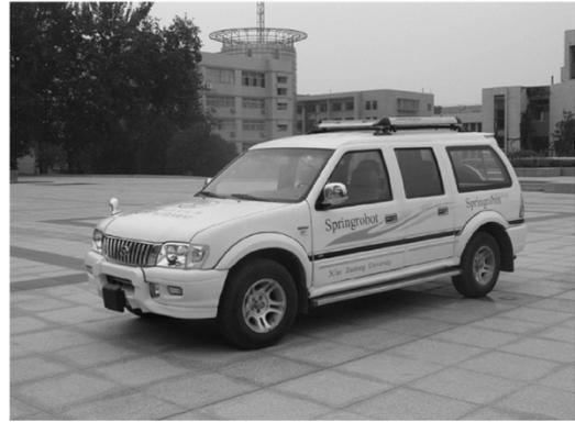
Fig. 1. Springrobot: prototype autonomous vehicle.
