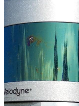
Fly splatters on LIDAR
