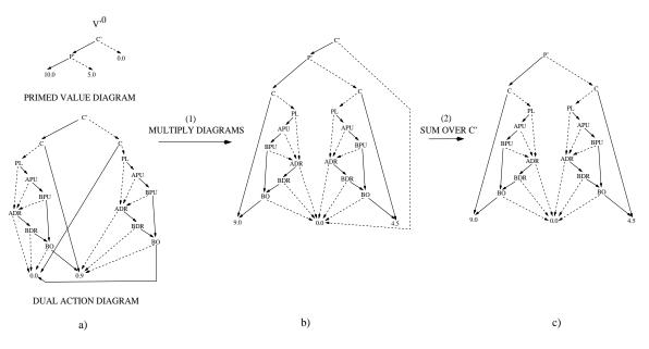
Figure 4: First Bellman backup for the *Value Iteration using ADDs* algorithm. (a) *0-stage-to-go primed* value diagram, and dual action diagram for variable C',  $Q_{C'}^a$  (b) Intermediate result after multiplying  $V^{\prime 0}$  with  $Q_{C'}^a$ . (c) Intermediate result after quantifying over C'.
