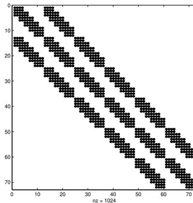
Figure 1: The structure of the QSC matrix arising from the discretization of a system of two PDEs subject to general boundary conditions with the alternating ordering, for  $N = M = 4$ . The number of non-zero entries is denoted by `nz`.
