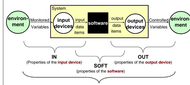
**REQ** (the requirements - relationships between monitored and controlled variables that the **system** is required to establish or maintain)
