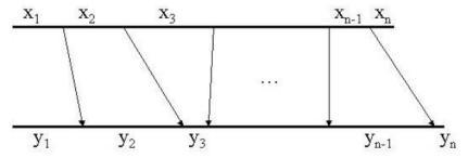
We will globally align X and Y by fixing the alignments of corresponding anchors to each other, and using NW to align the portions of X and Y between neighboring anchors.
