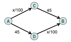
The meaning of the edge label "x/100" is that the time on that edge takes x/100 time units (e.g., minutes) if there are x people using that road. An edge label "45" means that it takes 45 minutes no matter how many people are using that edge. Drivers (commuters) have two possible paths to go from A to B. What route should they decide to take.
