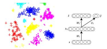
MNIST: nice clusters in the distribution  $\Rightarrow$  input distribution structure reveals the target class.  $f_1(x) = P(Y|x)$  related to  $f_2(x) = P(x)$ . Otherwise? combine supervised & unsupervised layer-wise greedy initialization. Add the two stochastic gradient updates (Bengio et al., 2007) Similar to Partial Least Squares EASY TO DO SEMI-SUPERVISED LEARNING WITH DBNs (Bengio et al., 2007)
