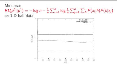
KL divergence w.r.t. epochs, b/w empirical  $p_0$  and (top) DBN trained greedily with CD, (middle) DBN trained greedily with  $KL(p_0||p_1)$  on the 1st layer, and CD on 2nd, (bottom) distribution  $p_1$  of 1st RBM, which should bound the other two curves.
