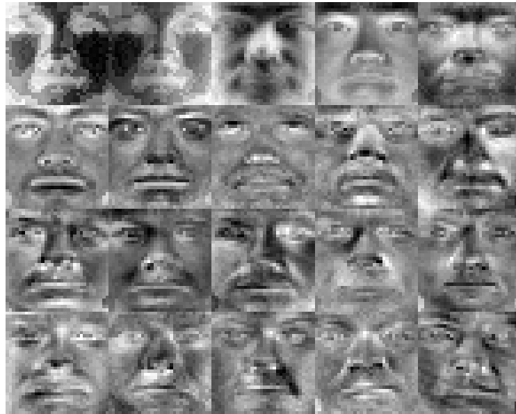
Fig. 16: The first 20 significant Eigenfaces of the selected face images, computed using the PCA algorithm.
