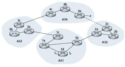
Suppose AS3 and AS2 are running OSPF for their intra-AS routing protocol. Suppose AS1 and AS4 are running RIP for their intra-AS routing protocol. Suppose eBGP and iBGP are used for the inter-AS routing protocol. Initially suppose there is *no* physical link between AS2 and AS4.
