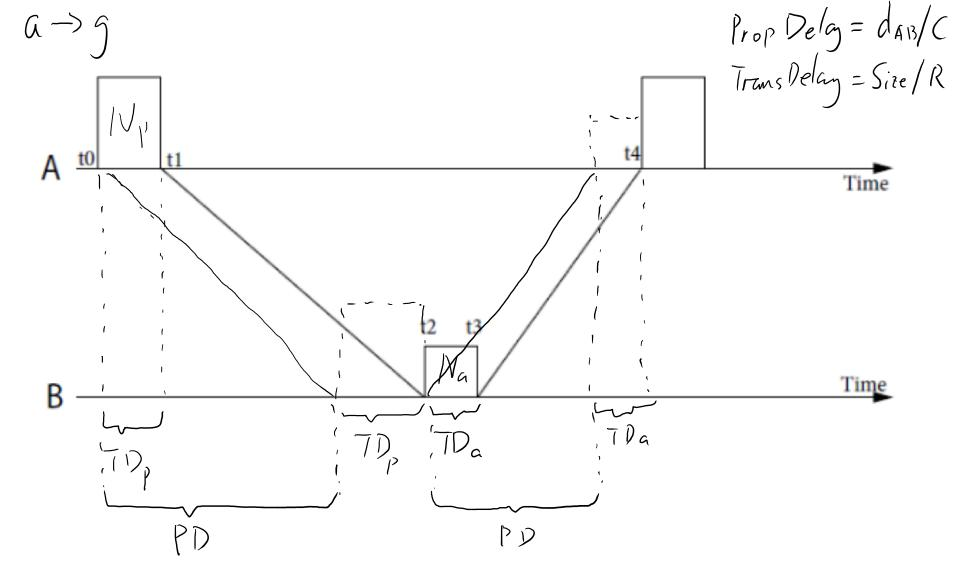
**d**)  $t_4 = t_3 + d_{AB}/C = t_0 + N_p/R + d_{AB}/C + N_a/R + d_{AB}/C = t_0 + (N_p + N_a)/R + 2d_{AB}/C$
