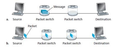
Consider a message that is  $8 * 10^6$  bits long that is to be sent from source to destination in the figure above. Suppose each link in the figure is 2 Mbps. Ignore propagation, queuing, and processing delays.
