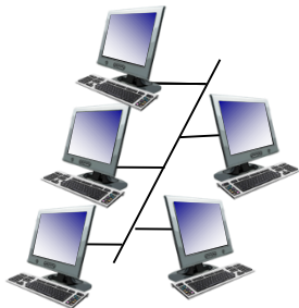
shared wire (e.g., cabled Ethernet)
