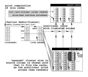
Figure 3. Projection Joins Using Partial Radix-Cluster
