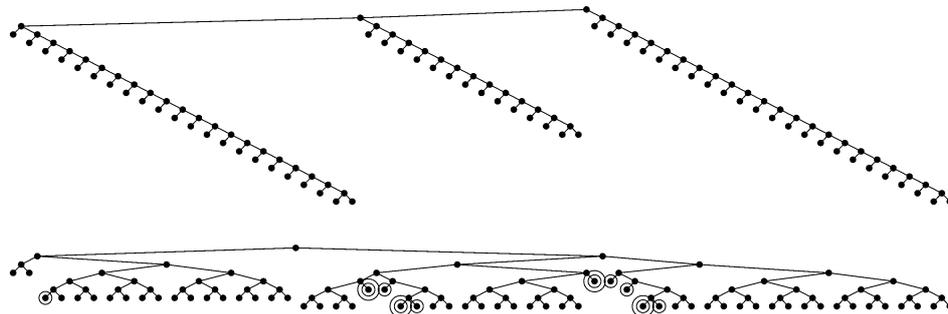
Fig. 7. Smallest tree (top) whose leaf-restricted  $h$ -leveling cost is 2 when  $h = \lceil \lg L \rceil + 1$  ( $L = 59$ ), and the resulting restructured tree (bottom) obtained by our algorithm. Leaves are circled a number of times equal to their depth increase.
