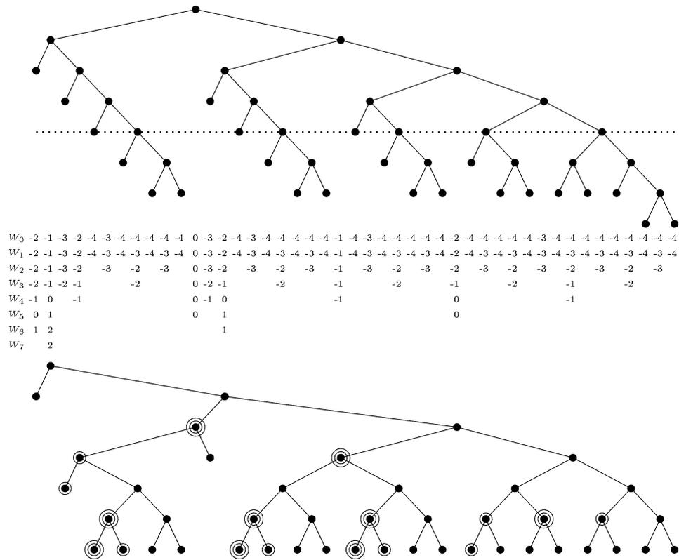
Fig. 9. An example of near-4-leveling, the resulting weight sequence, the weight sequences produced by the phased alphabetic minimax algorithm, and the resulting “balanced” tree. The original tree is a smallest tree ( $L = 23$ ) whose  $h$ -leveling cost is 2 when  $h = \lceil \lg L \rceil + 1$ . Nodes are circled a number of times equal to their depth increase.
