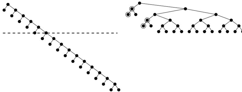
Fig. 6. Chain (left) with  $L = 16$  that is restructured (right) to have height at most 5. Nodes whose depth increased are circled.
