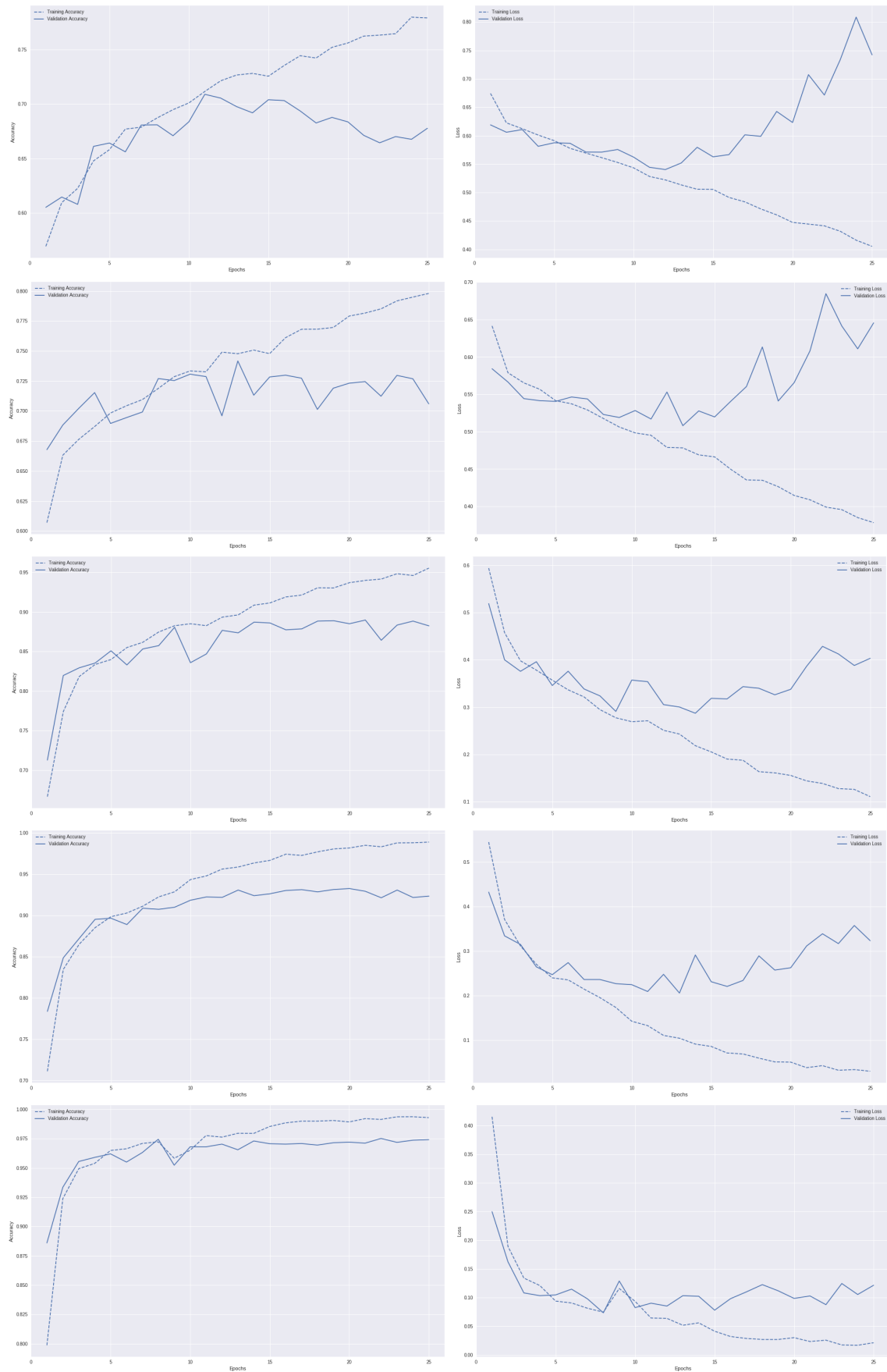
Figure 11: Training (dashed) and validation (solid) accuracy (left) and loss (right) metrics of neural network over 25 epochs trained using patches with nodules of radiodensity and diameter: (1) 30-150HU, 0.5-3cm (2) 30-150HU, 1-3cm (3) 350HU, 1-3cm (4) 500HU, 1-3cm , and (5) 1000HU, 1-3cm .
