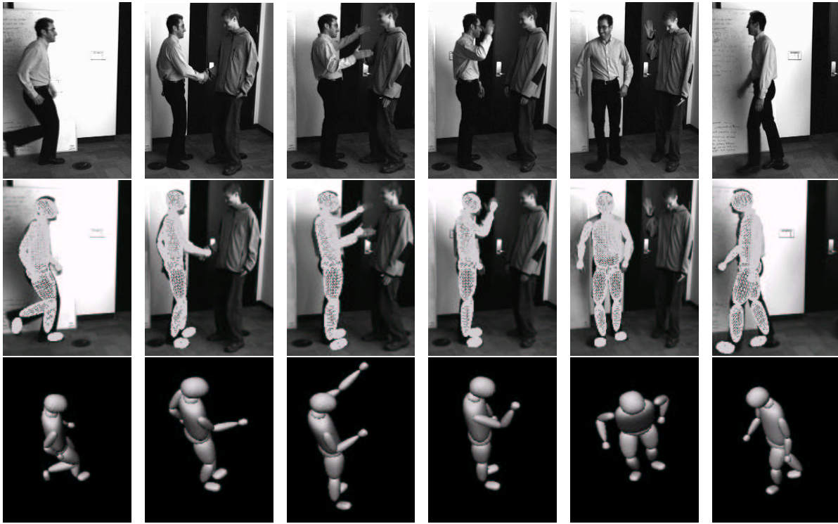
Figure 6. Tracking a 5s monocular video sequence of mixed running, walking and conversational activities over a 12d state space. Top row: original sequence. Middle row: most probable 3D model configuration (wireframe) projected onto image at given time-step. Bottom row: reconstructed 3D poses rendered from a synthetic scene viewpoint. Although clutter, motion variation and missing data resulting from frequent self-occlusion / disocclusion makes monocular tracking difficult, motion tracking and reconstruction have good accuracy. Without prior knowledge, the occluded limbs can't be reliably estimated.
