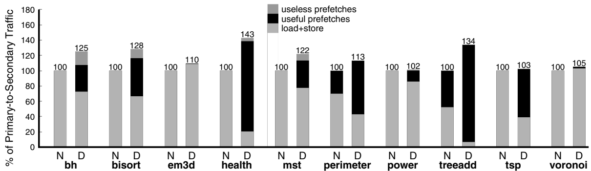
Figure 3.26: Breakdown of the traffic between the D-cache and secondary cache (N = no prefetching, H, H-A, and H2 are history-pointer prefetching schemes).
