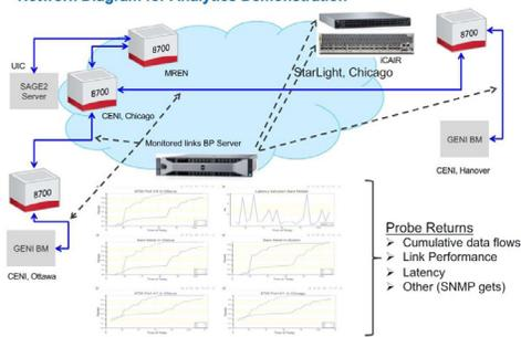
Ciena's CTO External Research Program has built an international testbed network connecting its Ottawa R&D facility to researchers in the United States and Europe. Through 2014 this Testbed was used for software defined networking (SDN), switching experiments, and demonstrations. Ciena Environment for Network Innovation (CENI) adds virtual cloud and compute resources to allow experiments in Network Function Virtualization (NFV) and protocols needed for distributed virtual infrastructures.
